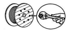
Due to changing weather conditions or transport, wooden drums may slightly shrink or loosen which necessitates retightening of the flange nuts.
